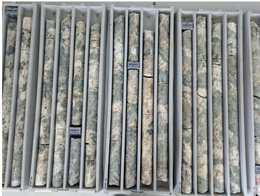
Figure 4. High-grade coarse grained spodumene (green) in drill core (FRDD01) from Grants.
