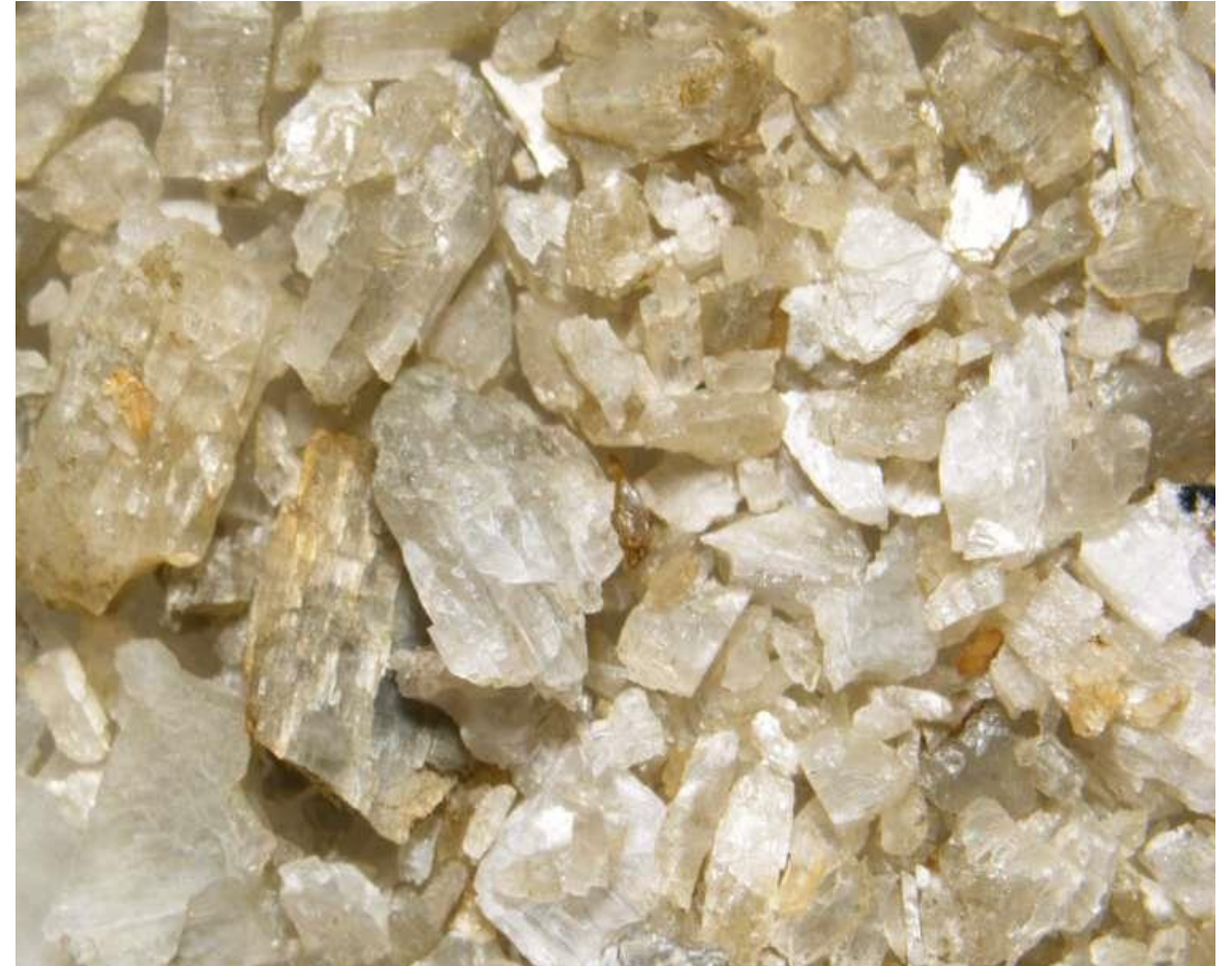
8.10% \text{Li}_2\text{O} Spodumene from HLS Testwork
