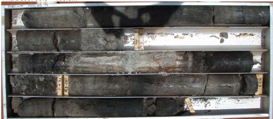
Photo showing a coarse grained, weakly oxidised light coloured sand unit constrained between reduced, fine to medium grained, sandy muds with lignite.
