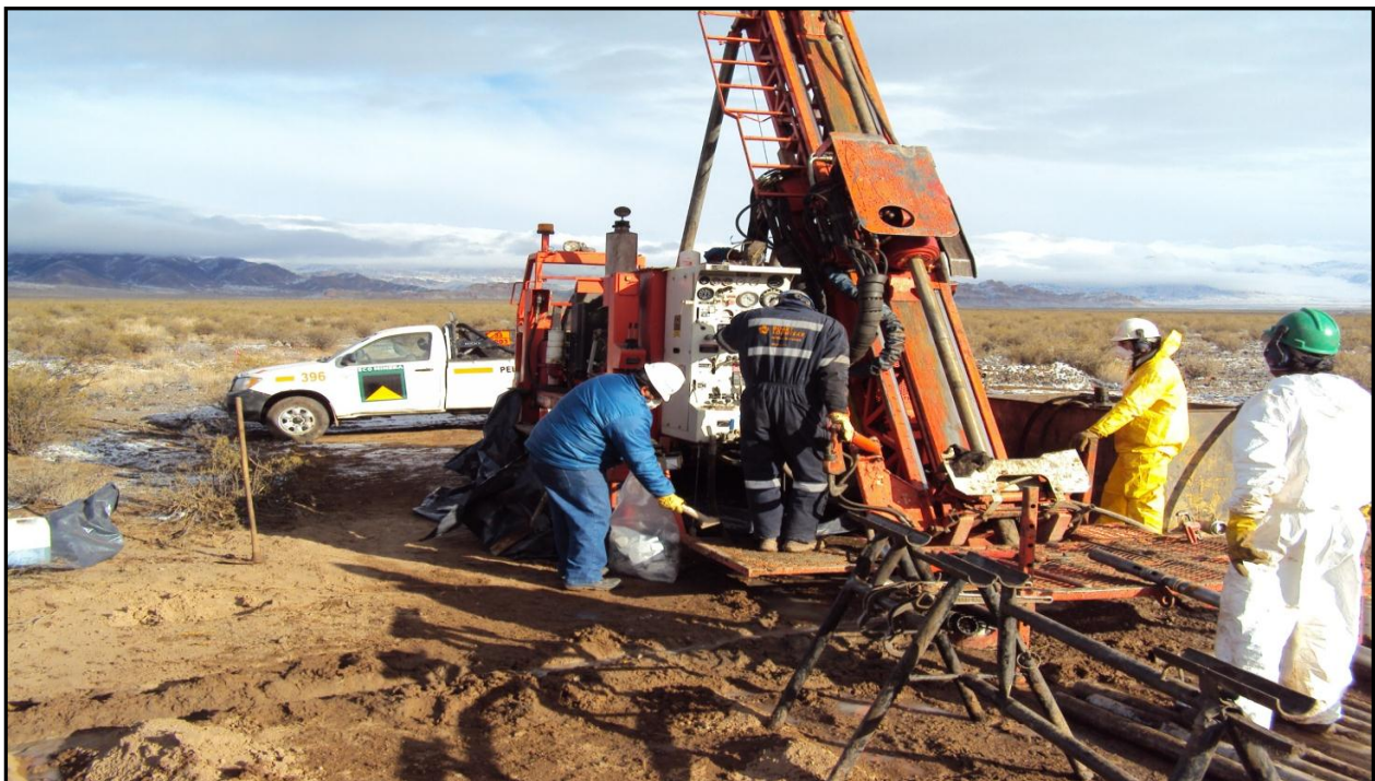
Diamond drilling at Las Marias Project, Argentina
