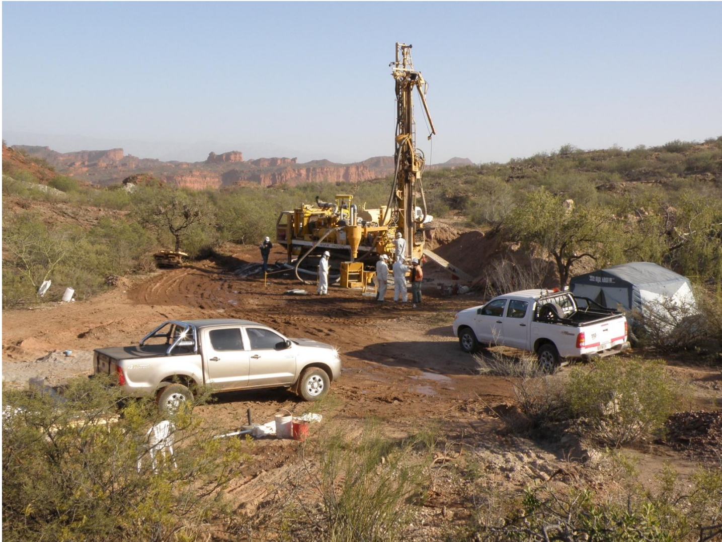
Figure 7: Los Colorados - reverse circulation drilling, August 2011
