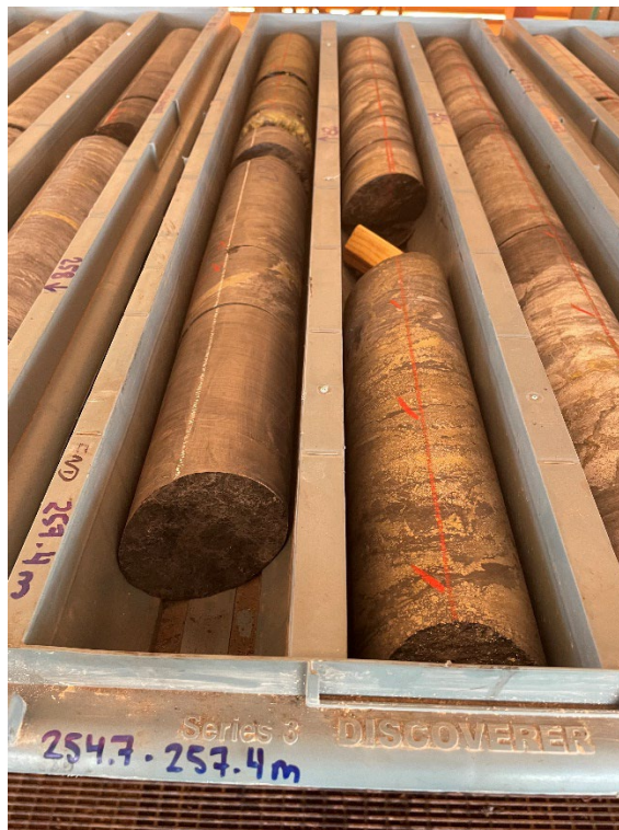
Figure 2-3: 23NFRCDM002 diamond drilled core, ~250m depth
