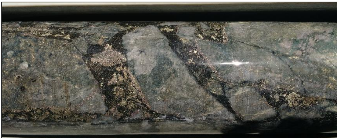
MGRCD001 – Tourmaline sulphide cemented breccia
