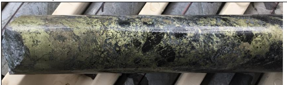
MGRCD004 – Sulphide cemented tourmaline breccia
