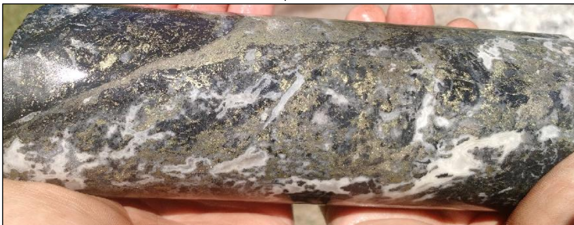
MGRCD001 – Quartz tourmaline carbonate sulphide breccia
