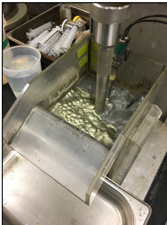
Figure 2: Photo – Flotation Concentrate Conditioning
