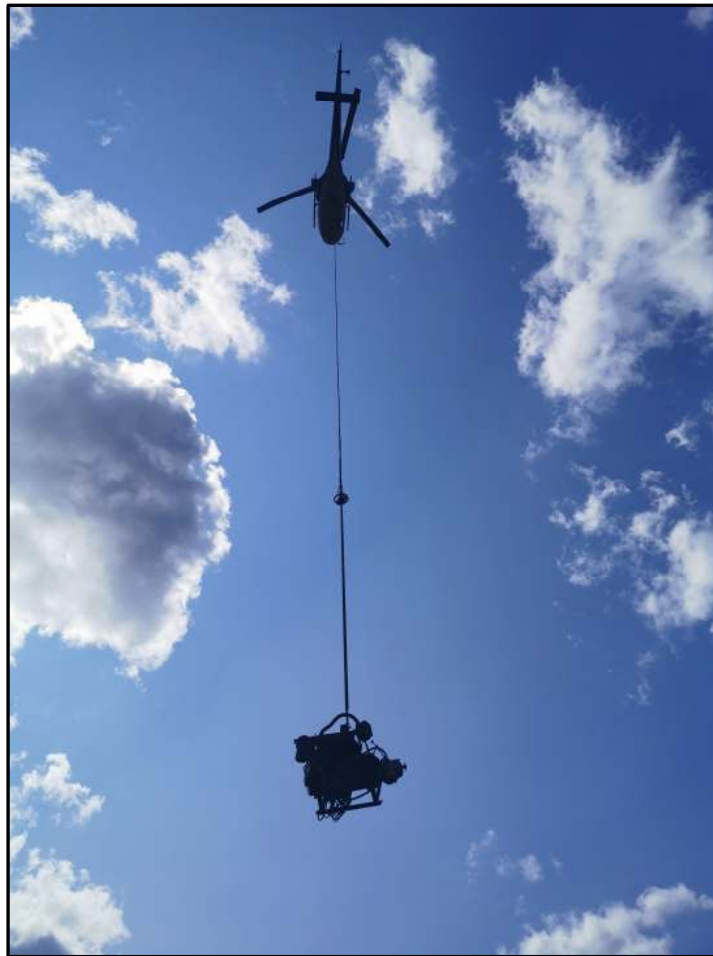
Figure 1 – Drill Rig En Route to Drill Site
