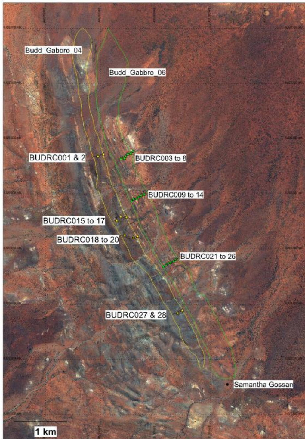
Fig 1 Location of the completed 2018 RC drill-holes with yellow triangles intersecting bands of massive and disseminated vanadiferous titanomagnetite in gabbro (Budd_Gabbro_04) and green triangles in the area of Budd_Gabbro_06 reporting vanadiferous magnetite in a mafic and felsic gneiss sequence overlain on high resolution Quickbird satellite imagery.
