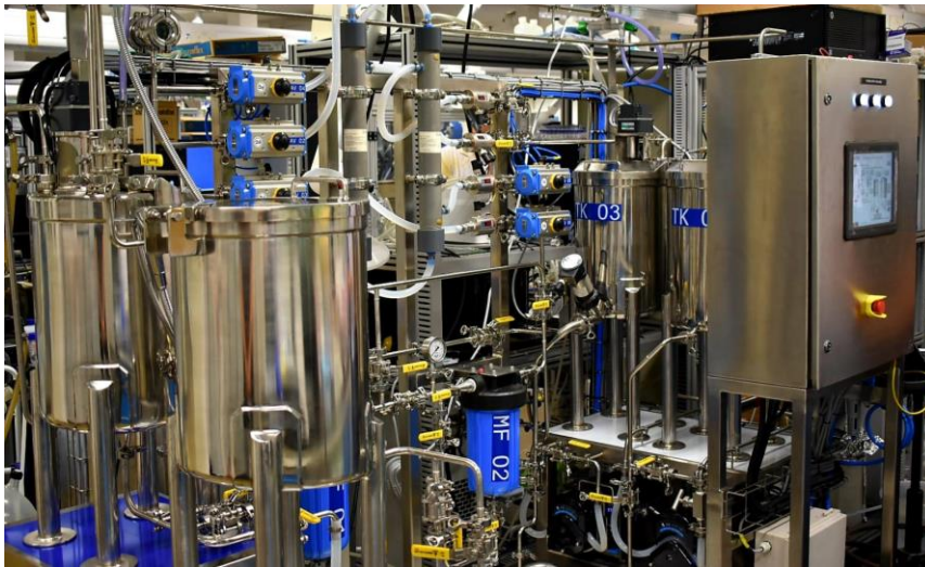
IMAGE 1) FO de-watering/liquid concentration system delivered by De.mem
