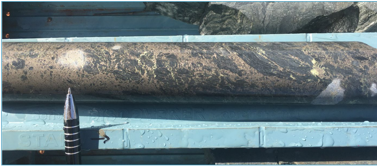
Semi massive pyrrhotite with chalcopyrite from 551.6m (Hole 20WD001). Gold mineralization is also associated with the copper.
