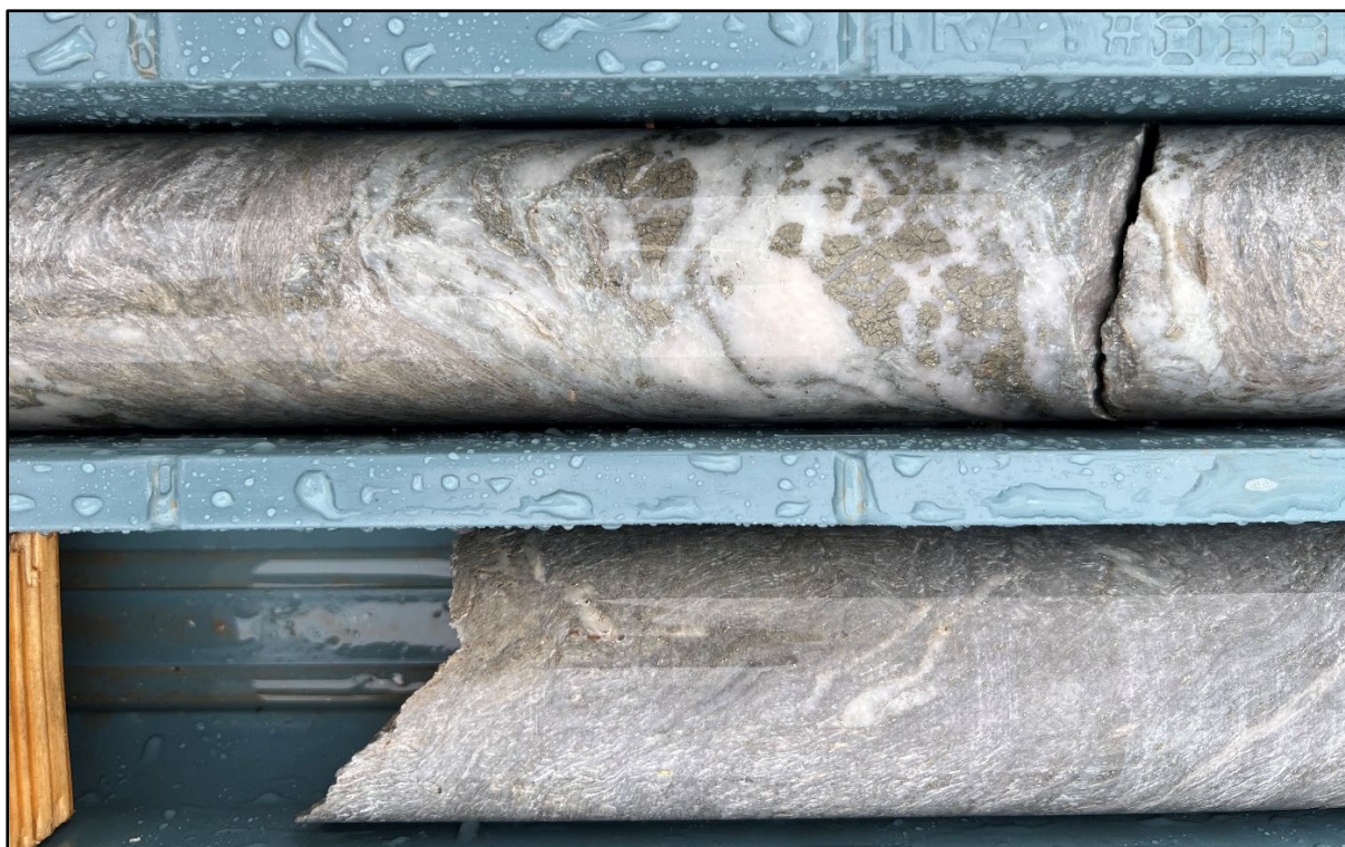
Figure 3: Nangus Road diamond hole 21JNDD001 close up of core at 300m (top) and 305m (bottom) showing pervasive silica, sericite, pyrite alteration with quartz pyrite veins.
