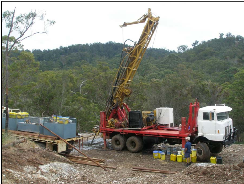
Figure 8: Drilling Diamond Core Hole ARD01 at the Amamoor Range Nickel prospect
