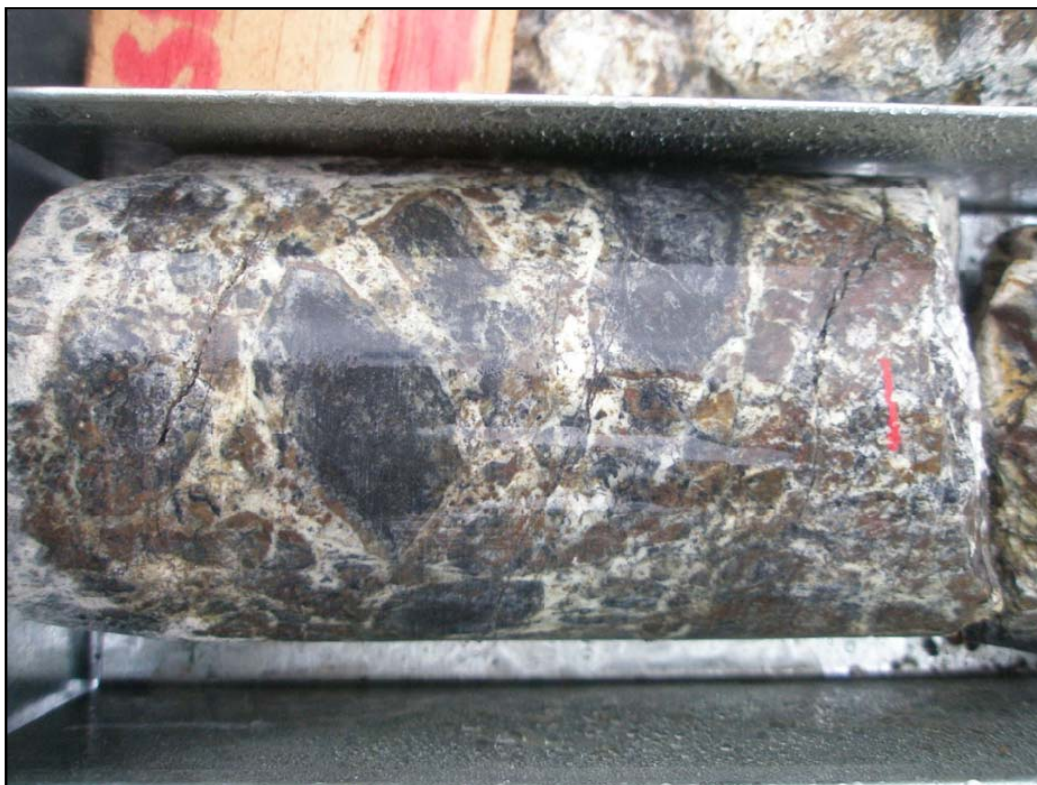
Figure 9: Near surface core from Amamoor Range, showing brecciated serpentinite with extensive magnetite veining (very similar to Mt Cobalt)
