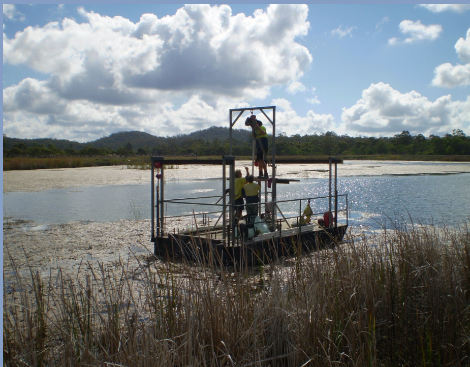
Figure 10: Drilling pontoon on the Shamrock Tailings Dam
