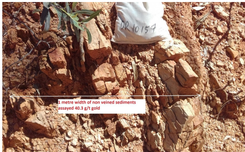
Figure 13: High grade gold in non-veined sediments - western section of Wally's Hope Prospect
