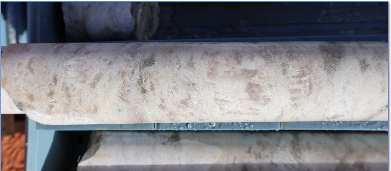
Figure 4: Coarse spodumene drilled by Red Dirt in YNRD005 at 129m.
