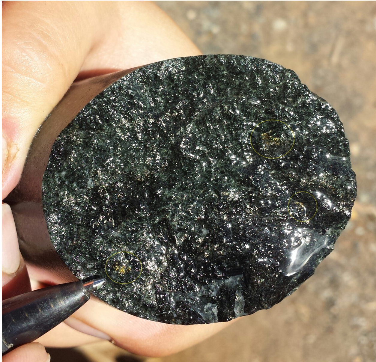
Figure 3 – Redback Prospect – One of the 12 visible gold occurrences identified within NQ2 drill core (diameter 50.5mm) from drill hole, SPDT010 at 207.28 metres. Three coarse clusters of gold circled in yellow with several smaller specks of gold scattered throughout broken core surface.
