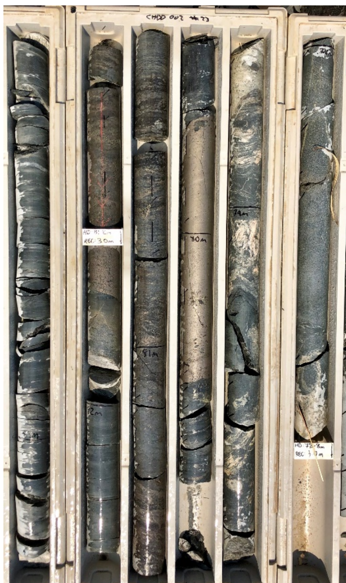
Figure 5: Massive and semi massive sulphides from the Upper Zone of CHDD002 with 79.8m-80.3m grading 1.9% Cu, 2.2% Zn, 1.0% Pb, 37.6 g/t Ag and 0.1 g/t Au
