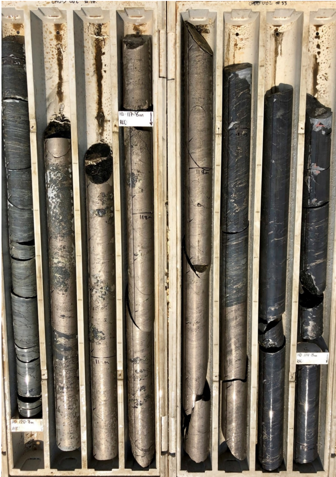
Figure 6: Massive sulphides in the Lower Zone of CHDD002 with 116.4m-120m grading 1.0% Cu, 4.9 g/t Ag
