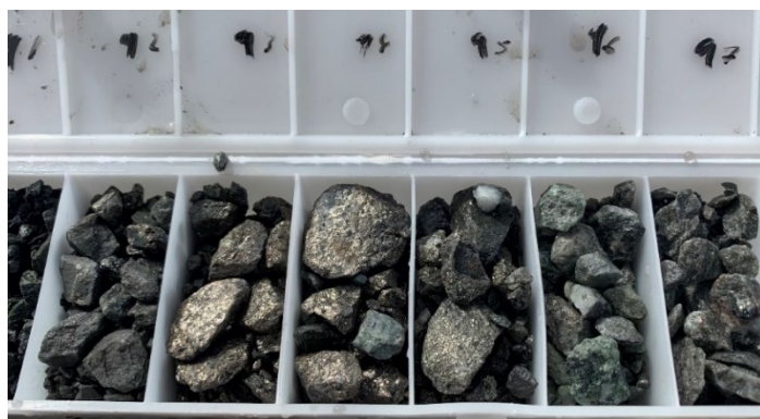
Figure 1: Chip tray from ILRC012 which was drilled into Warspite showing 3m of massive sulphide (>80% sulphide) from 92m, predominantly pyrite and pyrrhotite with trace (~1% visual estimate) chalcopyrite.
