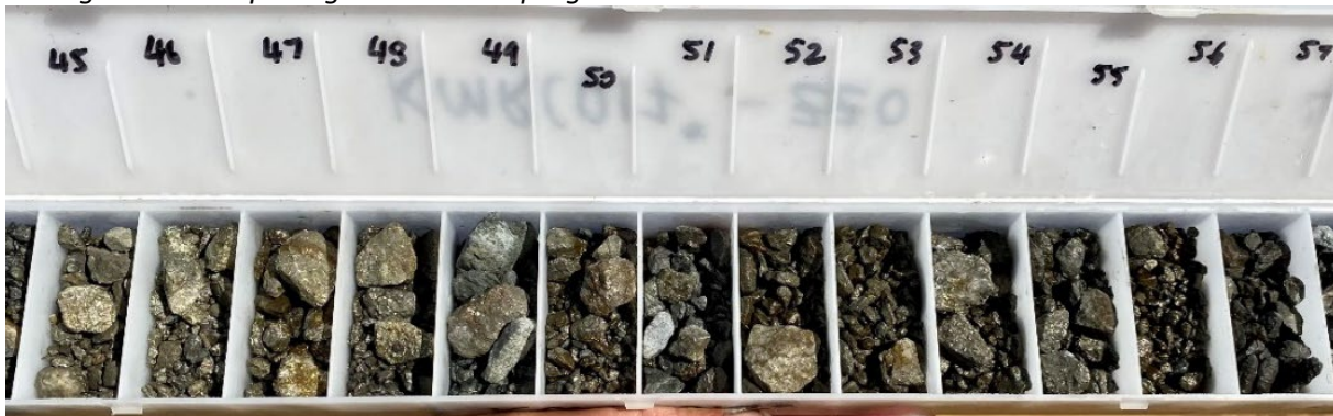
Figure 1: KMRC017 chip tray with semi-massive/massive sulphide (44-57m) carrying ~5-20% chalcopyrite.
