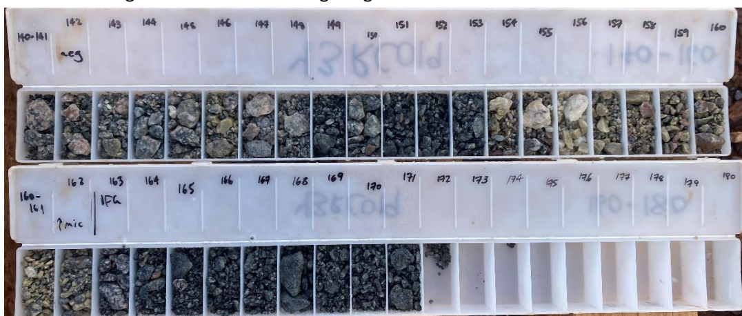
Figure 6: Chip tray from Y3RC019 showing dark fenitic alteration grading into two mineralised fresh ironstones (ferrocarnatite) from 142-163m.
