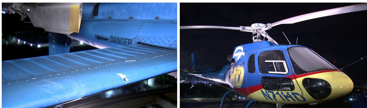
The LA News Helicopter that was struck by a drone at 1,100 ft AGL. The closeup image shows puncture damage to the wing caused by the collision
