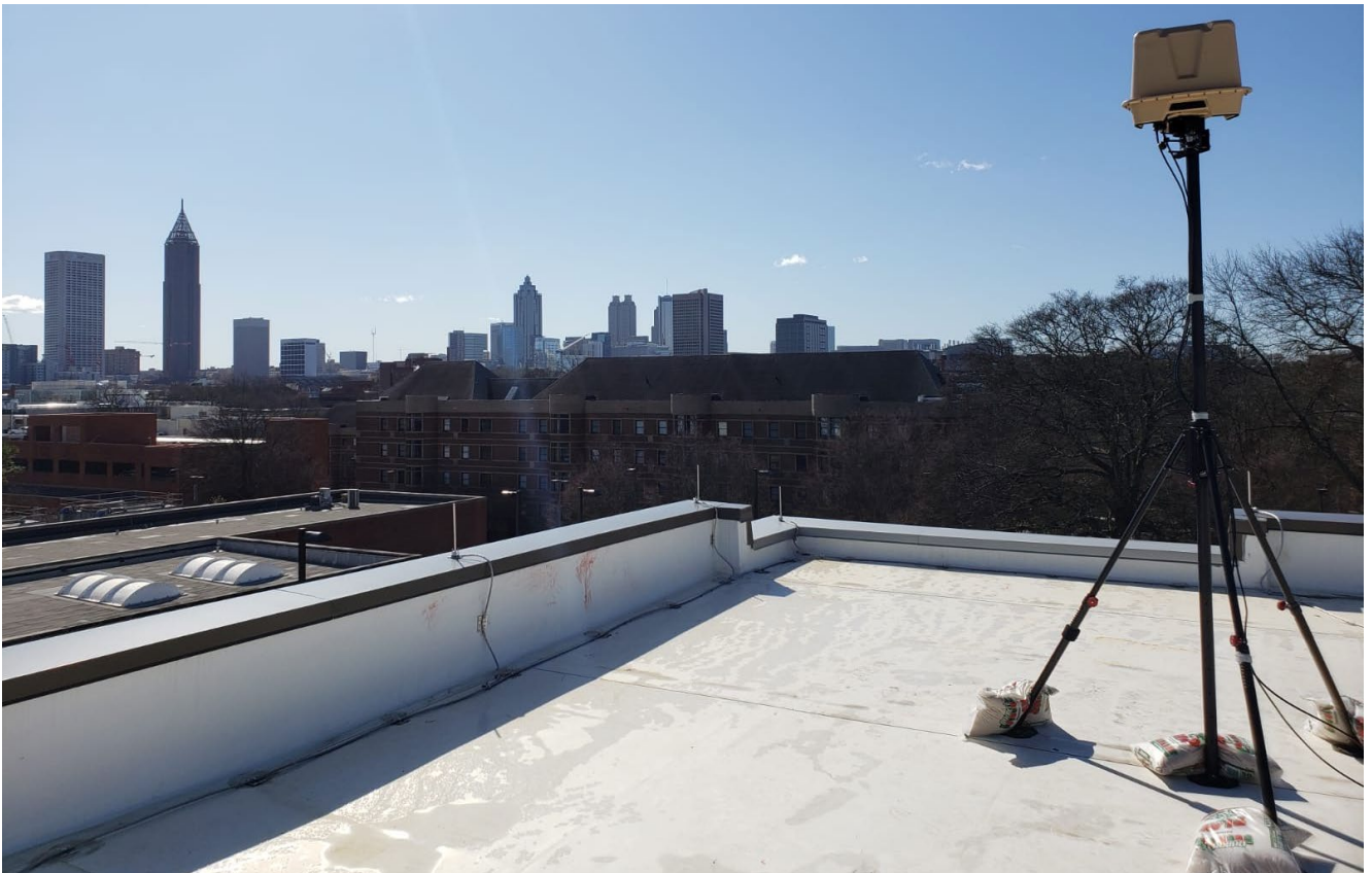
Image: DroneShield's RfZero – rapidly deployable, cost-effective and passive drone detector. Combined with DroneShield's proprietary DroneShieldComplete software suite, it can be used either as a permanent counterdrone solution, or as means for customers to "test drive" DroneShield products, and to understand the scale of drone incursions at customer sites.
