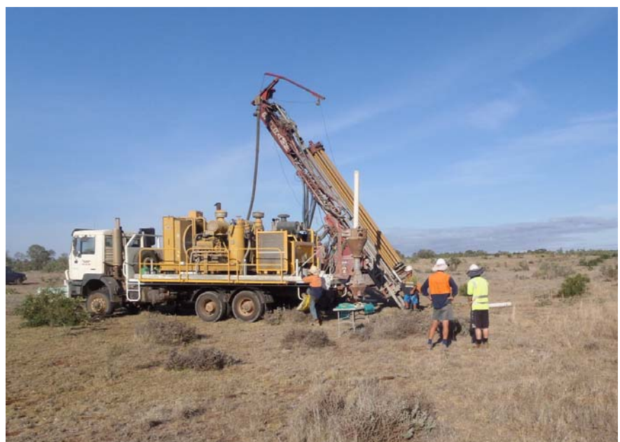
RC drilling in progress – Red Dog Prospect
