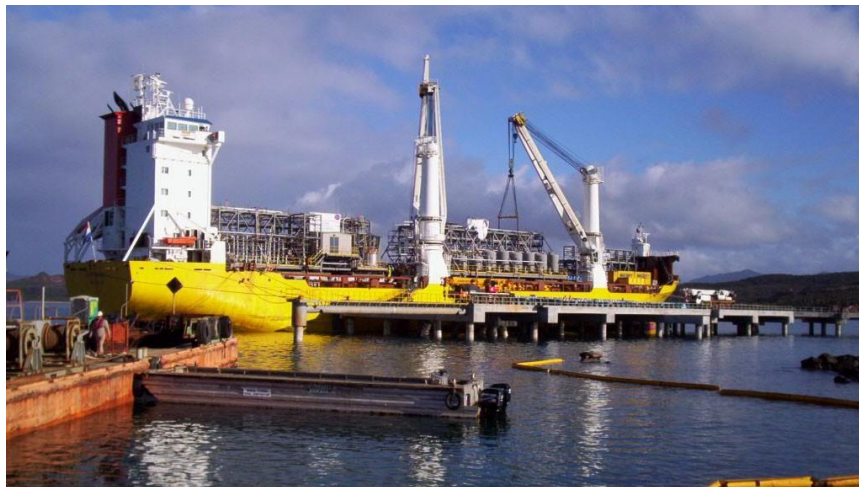
Figure 31: HLS transporting prefabricated modules
