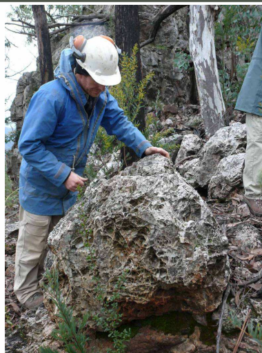
Unicorn Mo Silica Cap containing dense quartz stockwork with peak 1,380 ppm molybdenum
