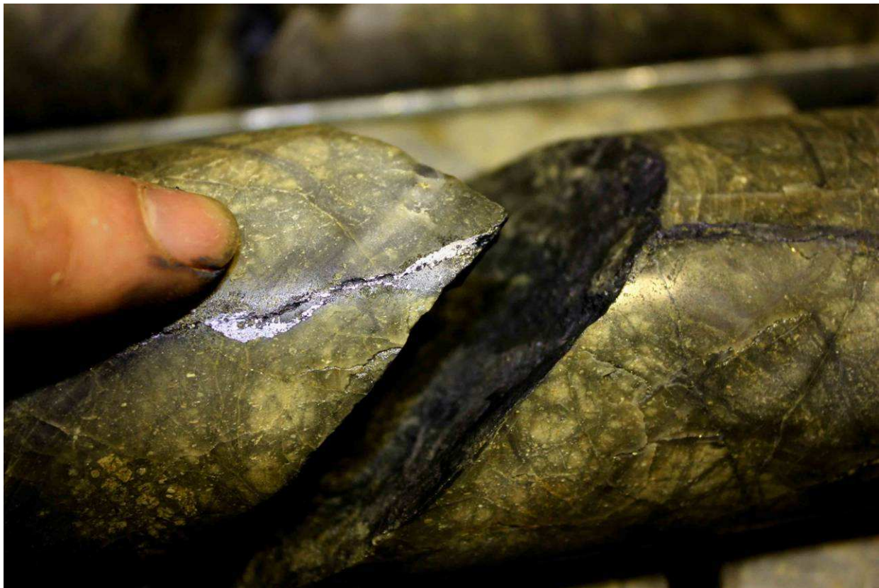
Photo 1: DUNDD004A – 249m. High Grade Molybdenite in a Radial Vein in altered porphyry.
