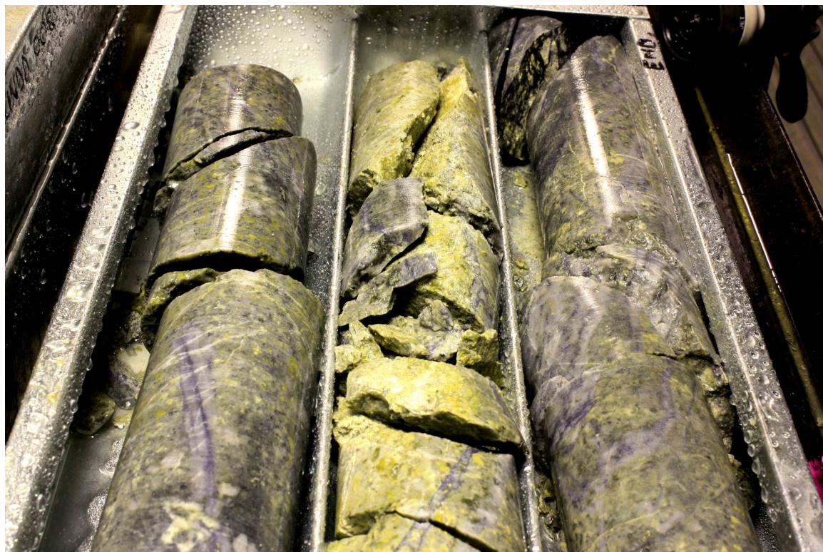
Photograph 1 DUNDD008. Visible molybdenum mineralisation (blue veins) in dense quartz stock work veins hosted by rhyolitic porphyry which is typical of the intersection between 340 – 387 metres.
