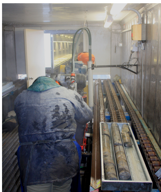
Photograph 5. Cutting drill core with a brick saw, strong suction fans remove mist and fine rock particles from the 6m converted sea container and roller tables ensure no lifting during the process of cutting 1000's of metres of core.
