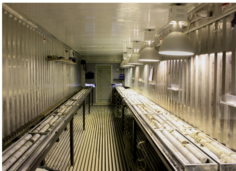
Photograph 4. Logging drill core within a 12m long converted insulated sea container, roller tables ensure no lifting of core trays throughout the logging, cutting and sampling process.
