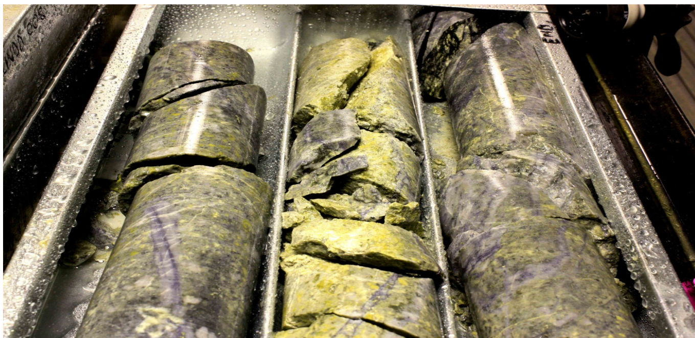
Photograph 1 DUNDD008. Average Mo grade of 0.08% over a 40 metre intersection (348 – 387.9m). Visible molybdenum mineralisation (blue veins) in dense quartz stock work veins which is typical of the intersection between 348-387.9 metres.
