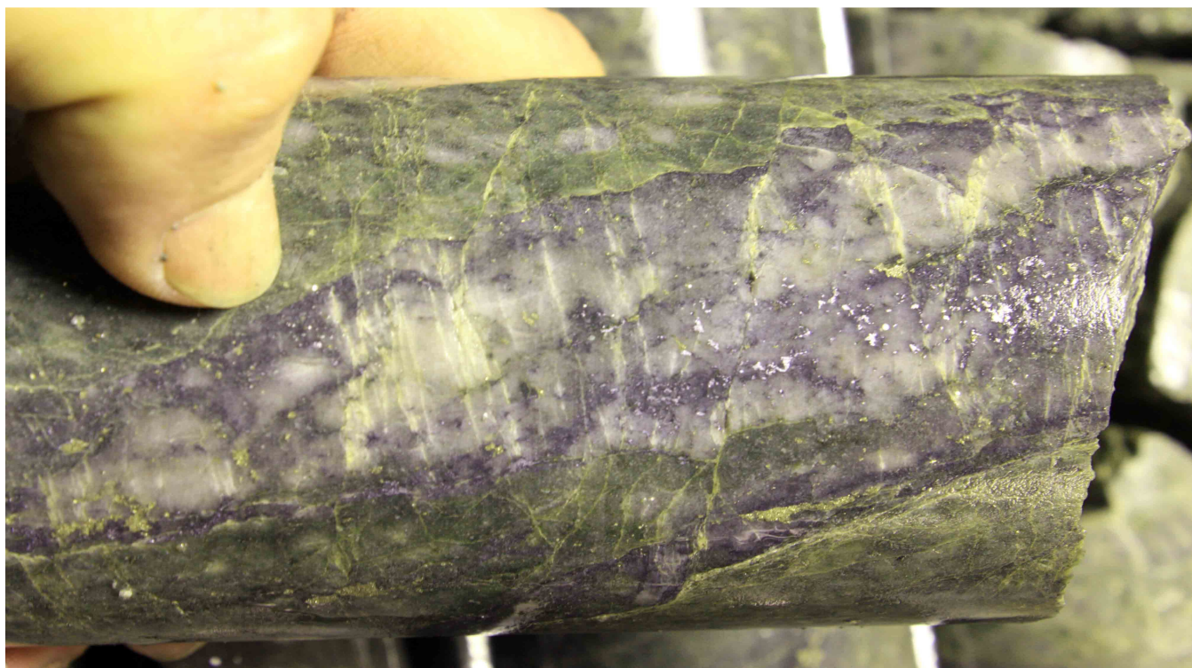
Photograph 3 DUNDD008. Example of strong coarse molybdenite mineralisation in quartz stock work veining – (Sample 100416: 2m @ 0.3% Mo and 29.1 g/t Ag – 368 -370m – Table 1)
