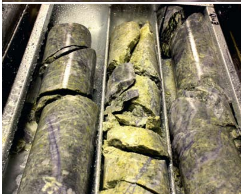
Top: Quartz-Molybdenite vein in porphyritic rhyolite host rock (DUNDD008) Above: Stockwork zone of quartz and molybdenite (DUNDD008)
