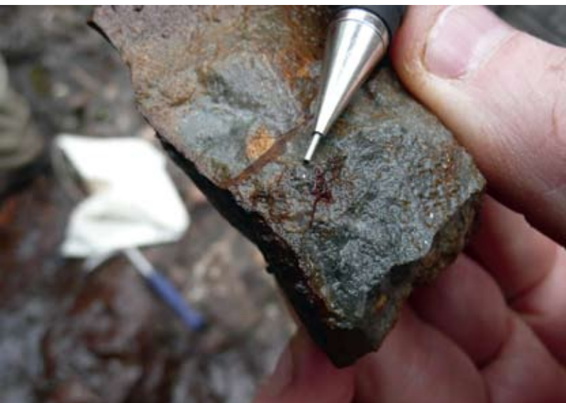
Visible molybdenite in brecciated sediments west of the October 2011 JORC Resource boundary.
