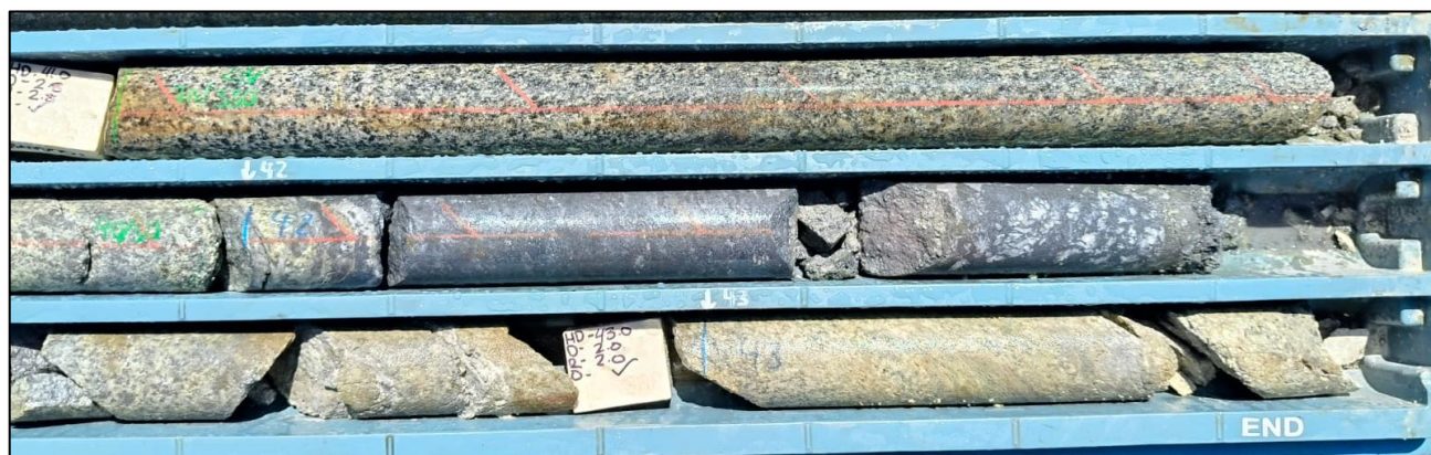
Figure 6: High-grade stibnite from 42m downhole in Drill Hole CBADD001, highlighted in red, assays 0.65m @ 32.20% Sb + 2.91 g/t Au + 10.50 g/t Ag within 5.0m @ 4.33% Sb + 1.69 g/t Au + 23.65 g/t Ag from 41.5m;
