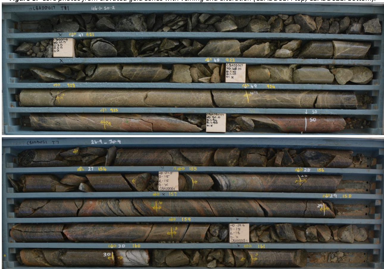
Figure 3: Core photos from elevated gold zones with veining and alteration (CBADD017: top, CBADD021: bottom).
