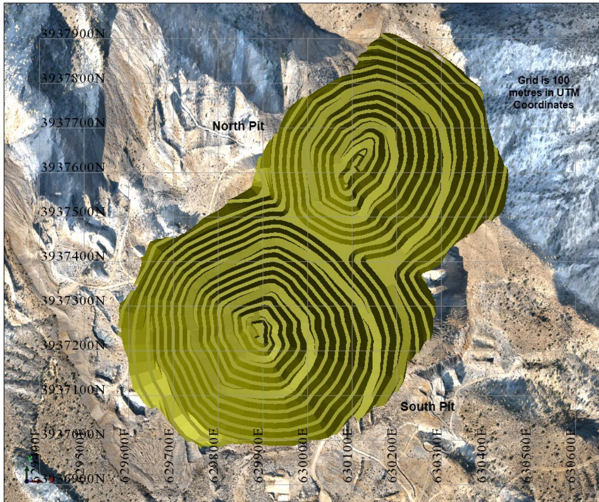
Figure 40 Final Open Pit Design
