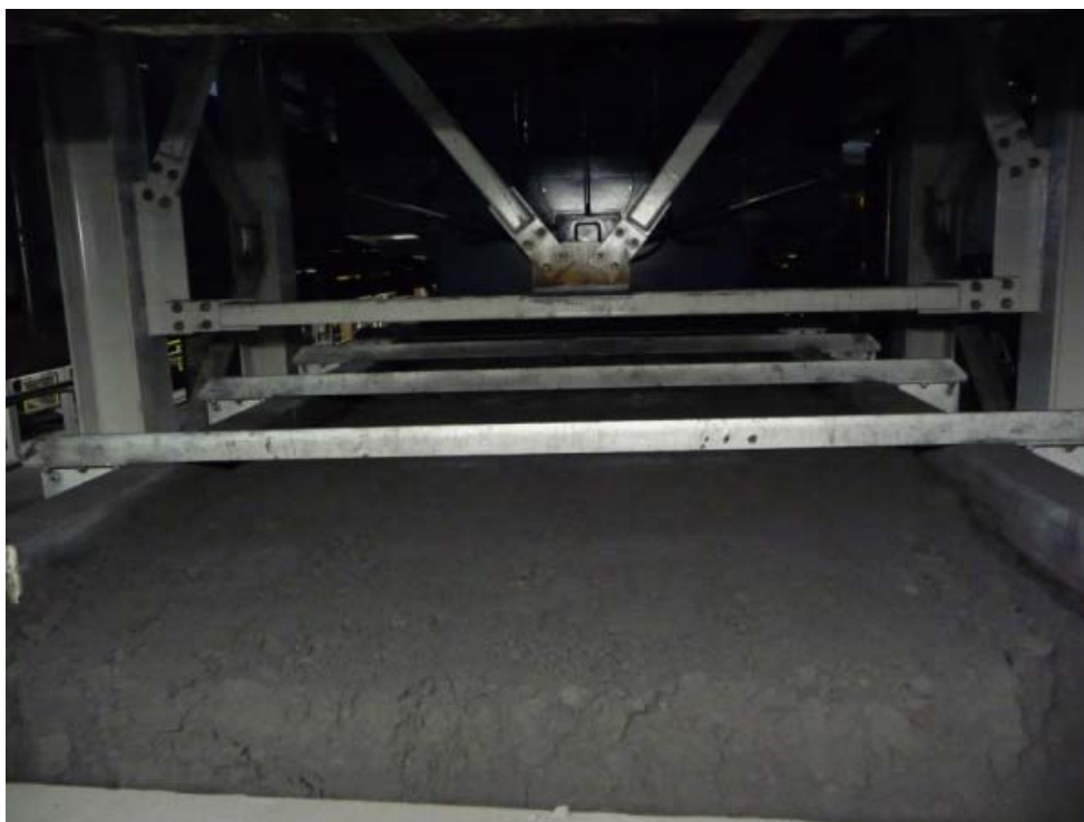
Figure 5 - sub 7% moisture concentrate produced by the filter
