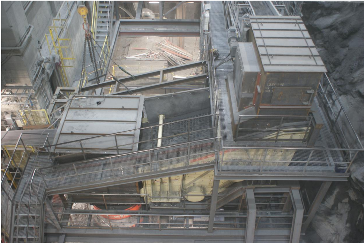
Figure 1 - new secondary crusher pre-screen in operation at Sydvaranger
