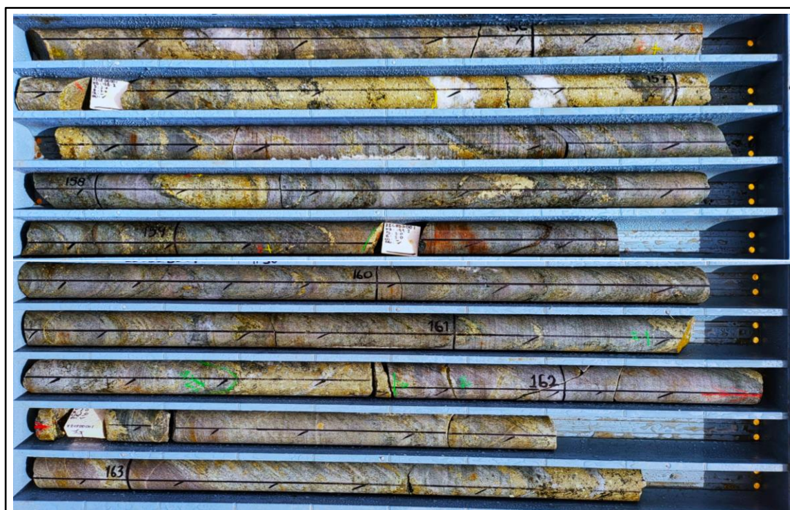
Figure 2: 22CEDD001 drill core 154.6m-163.9m, massive and semi-massive sulphides
