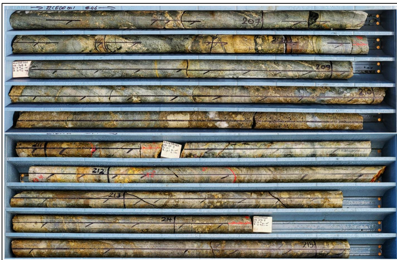
Figure 3: 22CEDD001 drill core 208.2m-215m, massive and highly disseminated sulphides
