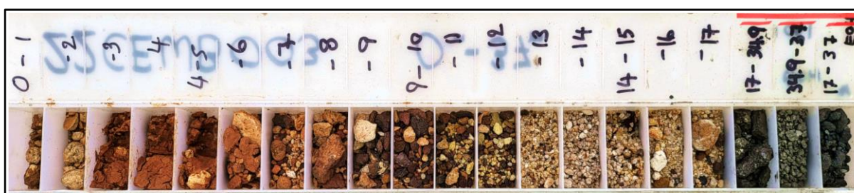
Figure 8: 22CEWB003 drill chips from 0m to end of hole (37m). For details of this drill hole refer to ASX announcement dated 26 September 2022.
