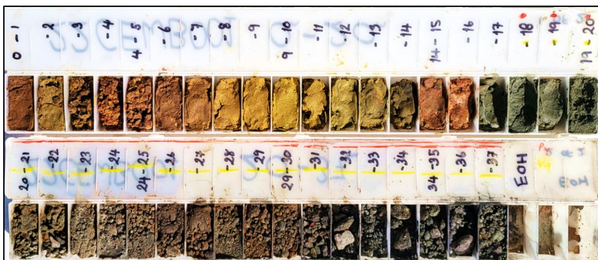
Figure 7: 22CEWB001 drill chips from 0m to end of hole (37m). For details of this drill hole refer to ASX announcement dated 26 September 2022.
