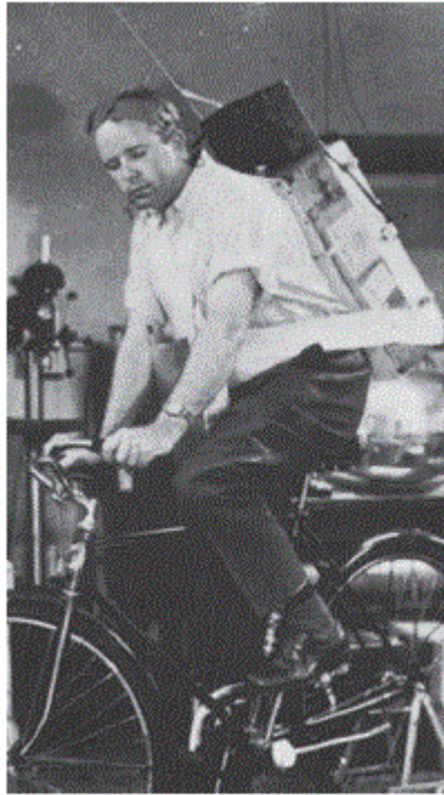
Figure. Jeff Holter with his original 38-kg radio-electrocardiograph recording device in 1947.
