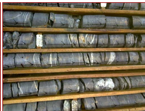
Photo 2: Altered and veined sediments, drillhole 09JTDD003.
