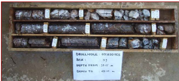
Photo 1: ferruginous breccia from drillhole 09SEDD005.
