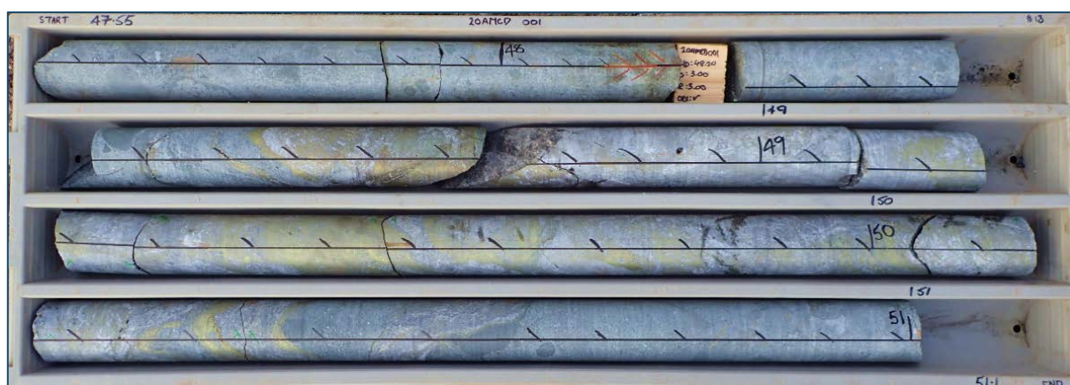
Figure 1: Semi-massive to stringer chalcopryrite mineralisation within chlorite altered fragmental rhyolite in 20AMCD001.
