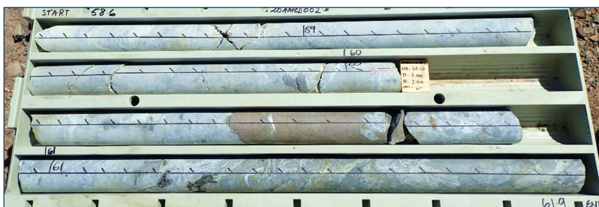
Figure 2: Massive sphalerite-galena mineralisation grading into a semi-massive to stringer zone within the upper chert horizon from 60.5m in diamond drill hole 20AMCD002.
