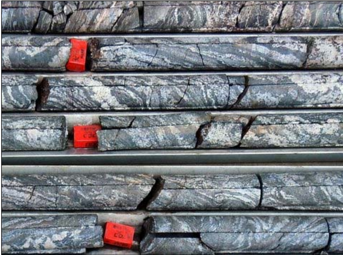
Figure 12: Shiyela Iron Project M63 – Medium to coarse-grained dark grey magnetite bands at 23 metres depth (Hole SHID4)
