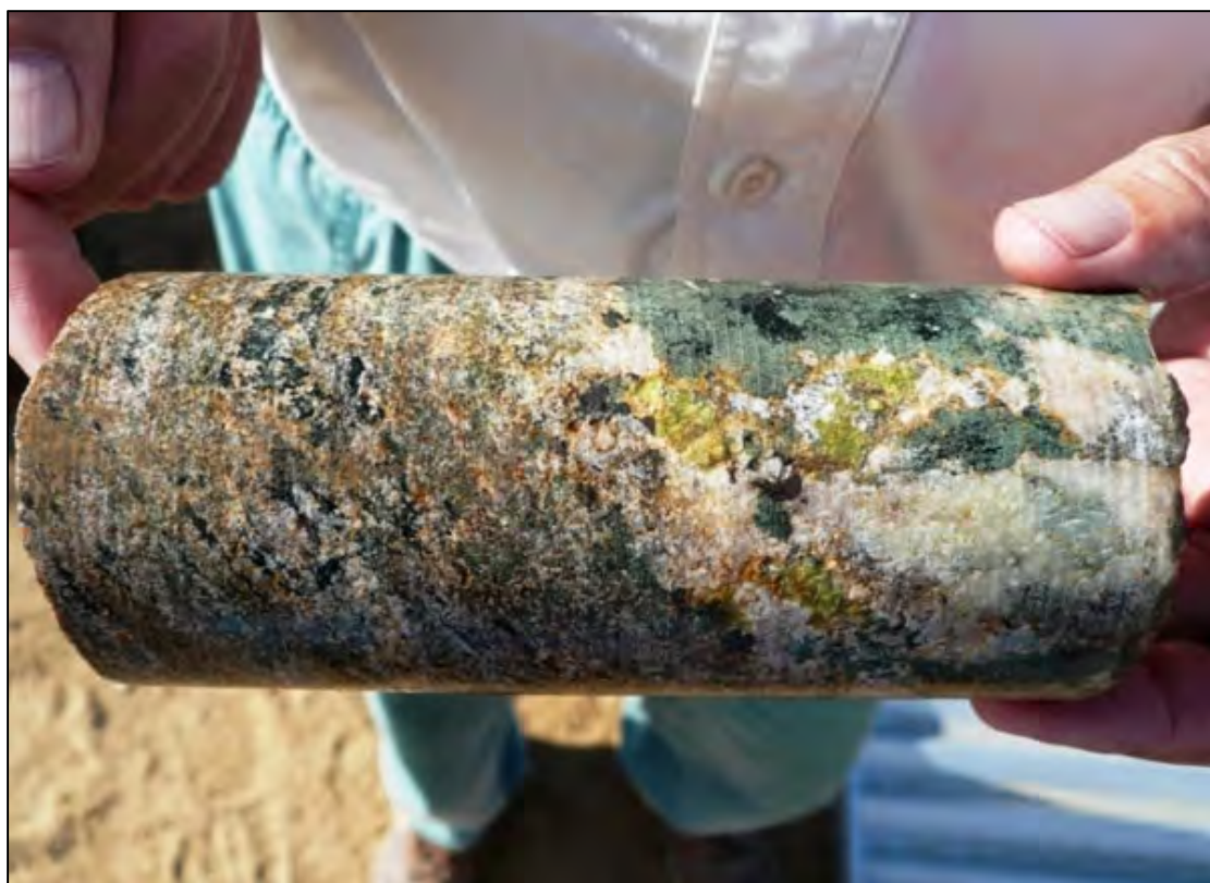
Figure 5 HQ diamond drillcore – altered granitic host rock with black magnetite, skarn alteration and yellow-green secondary uranium mineralisation (uranophane and beta-uranophane)
