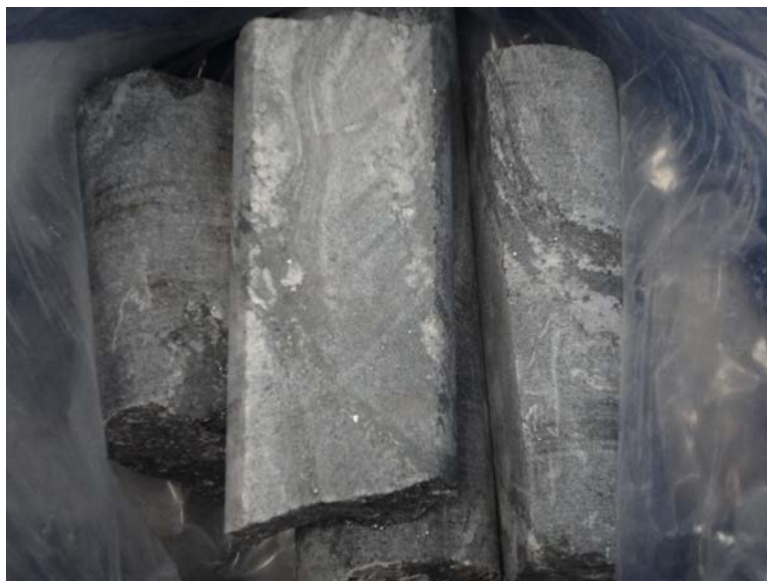
Figure 3: Shiyela PQ Core Showing Hematite
