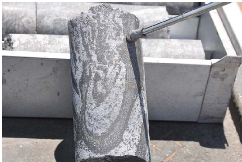
Figure 4: Shiyela PQ Core Showing Folded Magnetite Bands
