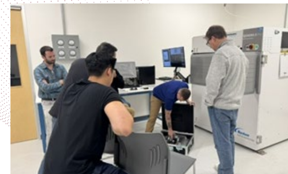
New x-ray machine for inspecting sealed assemblies
