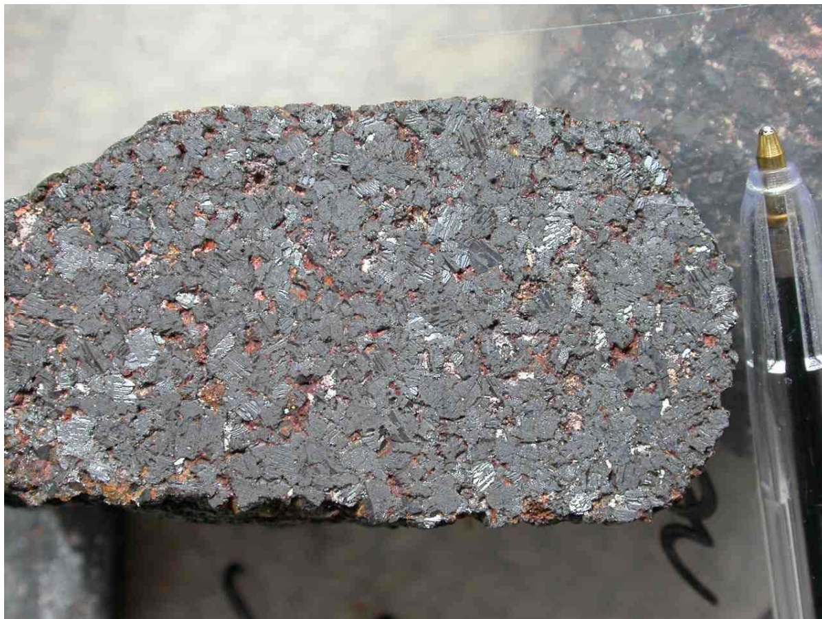
Figure 3: Slabbed surface sample of massive coarse magnetite from Hawkwood.
