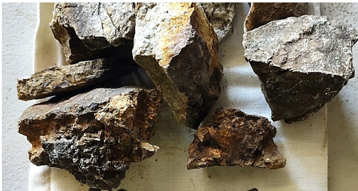
Figure 4: Sample 3017023, best Au sample (12.3ppm) has narrow zones of gossanous breccia (lower) with anomalous Cu Ag Bi Mo S in albite altered porphyry (upper).
