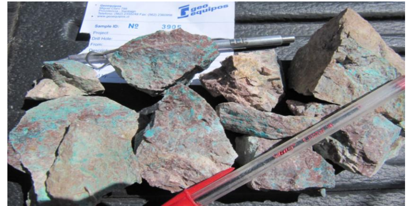
Selective samples assayed 1.59% copper & 0.6g/t gold (left), and 1.47% & 0.69% copper (right)
