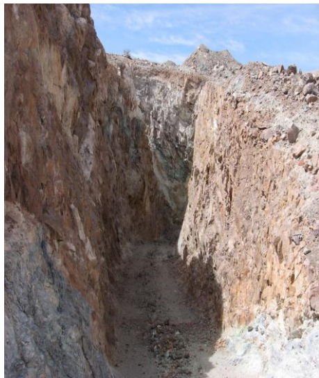
Selective samples assayed 1.59% copper & 0.6g/t gold (left), and 1.47% & 0.69% copper (right)
