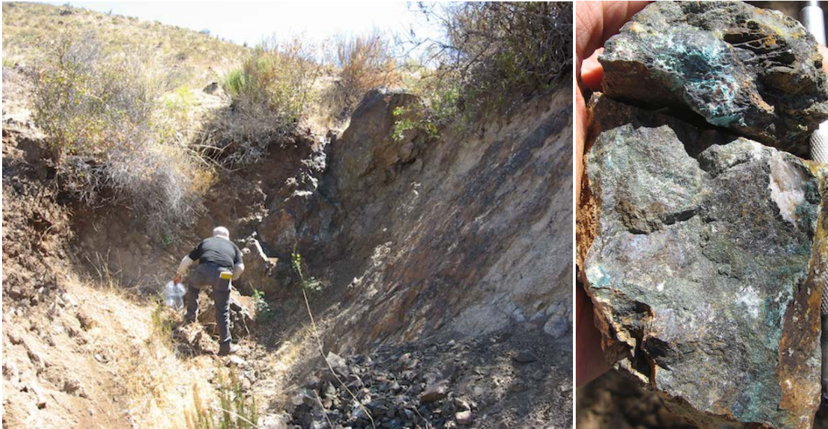
Figure 4: Vein structure on eastern flank being sampled (left) and material from the vein (right) composed of quartz, calcite, copper oxides, sulphides, pyrite and limonite. Sample 954523 returned grades of 1.88% copper and 0.29 g/t gold.
