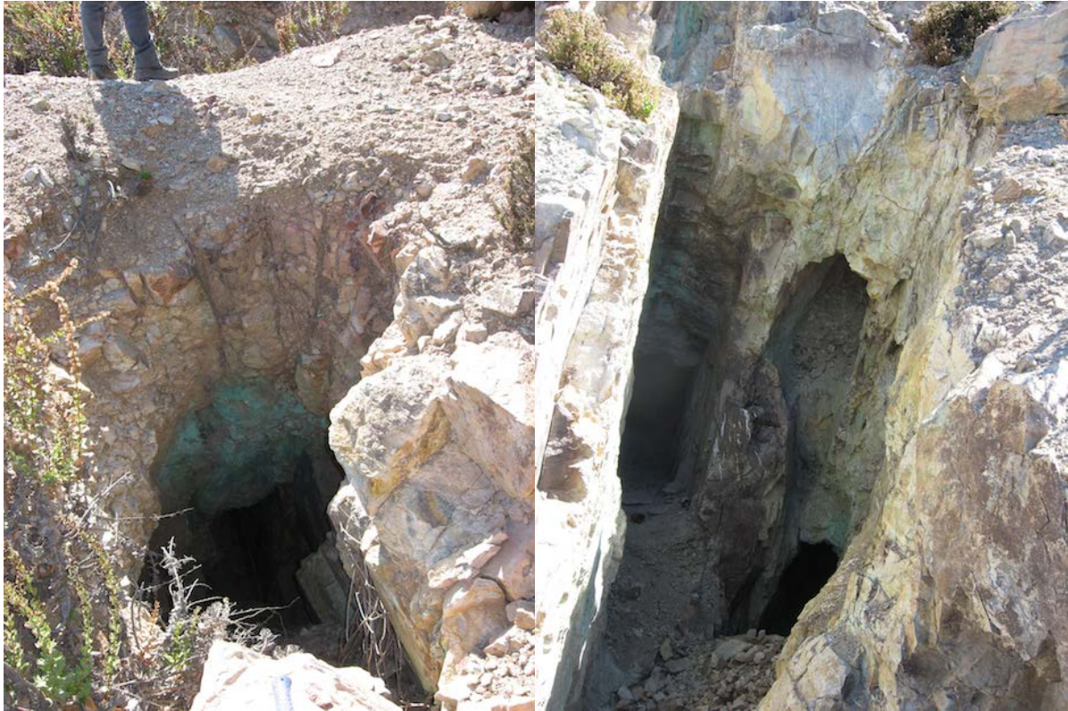
Figure 6: Fracture/fault zones on the western flank of the Tamaya hill hosting mineralised veins that have been worked to a shallow depth. Sample 954529 (left) reported grades of 1.52% copper and 0.05 g/t gold. Sample 954530 (right) reported 3.02% copper and 0.16 g/t gold.
