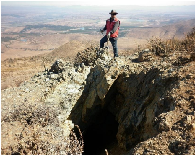
Channel sampling across a working on a sub-parallel vein some 550 metres to south of the other sample points. The two metre wide sample assayed 2.25% copper
