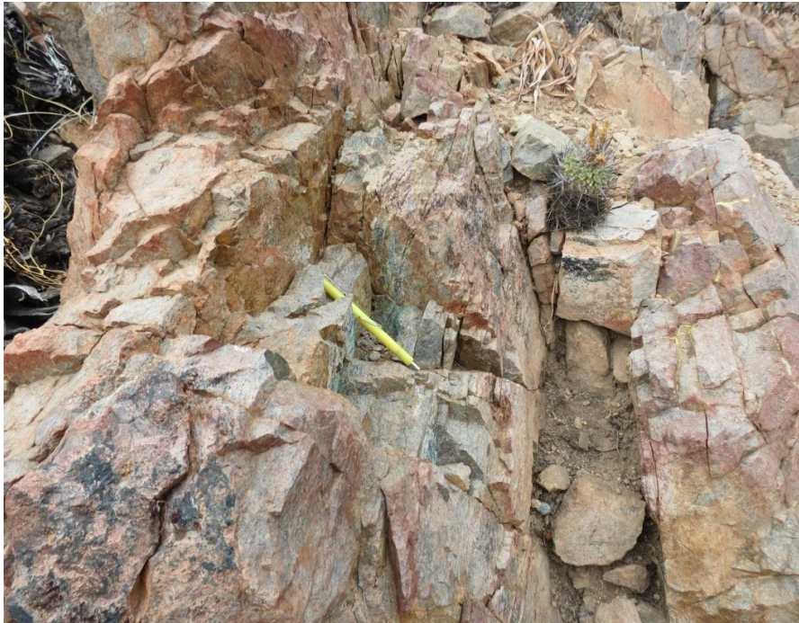
Potassic alteration with magnetite overprinting the rhyolitic dome. The dome is strongly fractured locally and returned a grade of 3.53% copper
