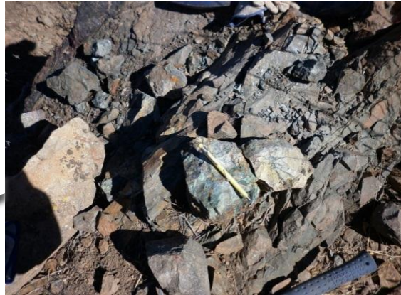
Two metre channel sample from the 110 metre long structure shown to the left, taken over a width of two metres with 1.57% copper
