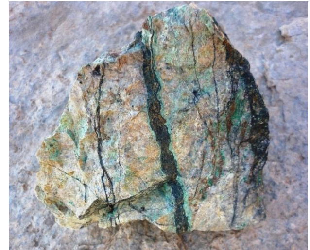
Rhyolitic wallrock to the Almagre mine on the main vein, with 0.98% copper
