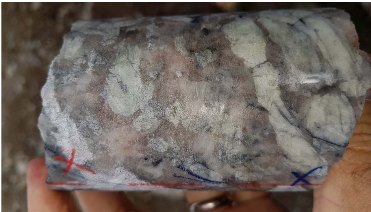
Figure 10: Hole 10 in the northern pegmatite which intersected 7 metres at 1.36% \text{Li}_2\text{O} from a downhole depth of 15 metres (vertical depth of 12 metres) including, 2 metres at 2.24% \text{Li}_2\text{O} from 17 metres;
